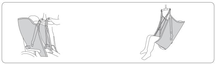
**Tip:** Check that all suspension loops have the same length, i.e., are at an equal height when they are stretched prior to lifting. Adjust the position of the sling if they are not at an equal height.
